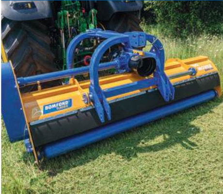
Hydraulic side shift Hydraulic offset function on all models.
