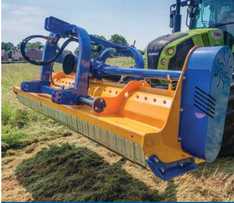
Easy adjustment Drive belts protected, heavy duty skids supplied and front steel flaps.
