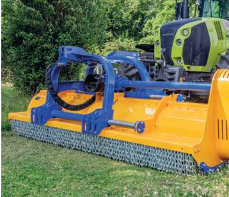
Chain guard protection Heavy duty chain guarding to protect against debris being thrown from the mower.
