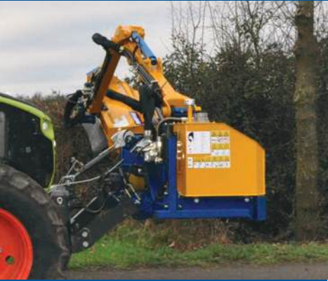
Covered hydraulics A powerful 104 litre system creating 60hp.
