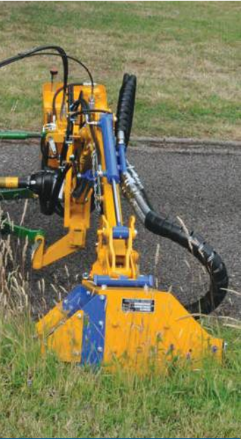
Gravity breakout system For protecting drive and machine during operation.
