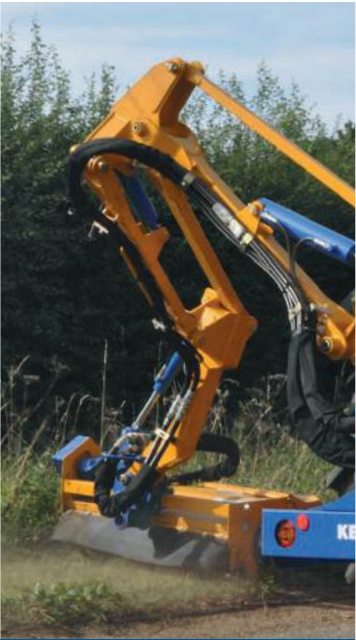
Clear visibility Variable forward reach brings cutting head into drivers view.
