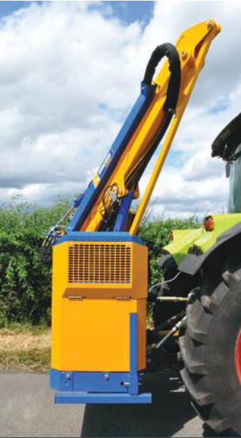
Slimline compact transport position Keeping weight closer to tractor for faster road speeds.
