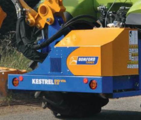
Low profile tank Aids driver visibility.
