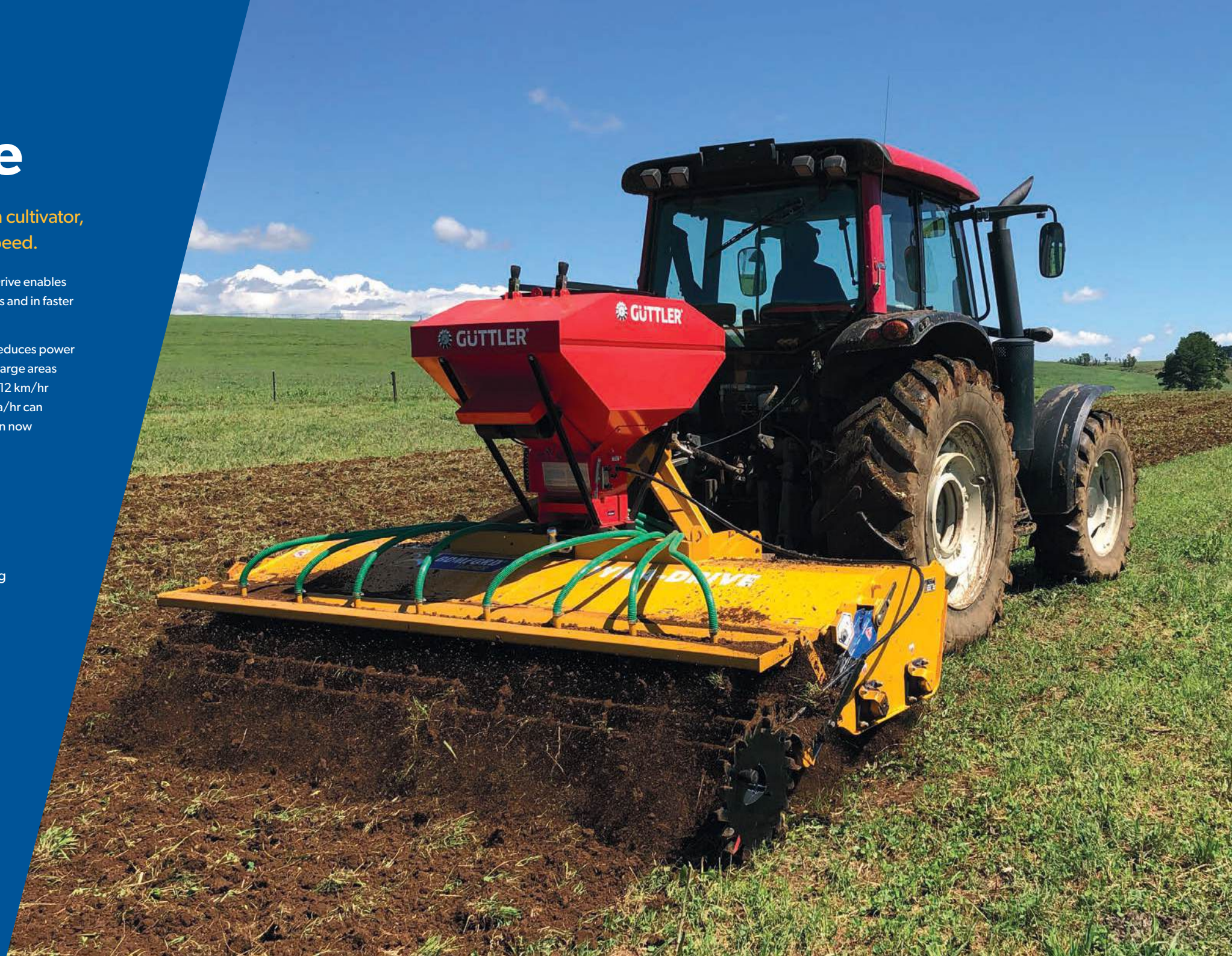
Dual rotors Two rotors connected via a single drive.
