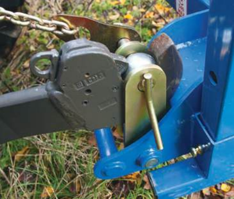
Mechanical breakout For machine and operator safety.
