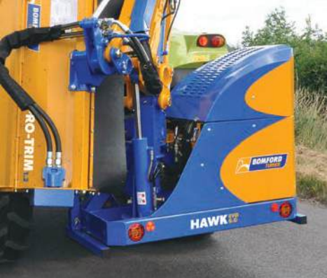
Fully enclosed hydraulics Keeping components protected.
