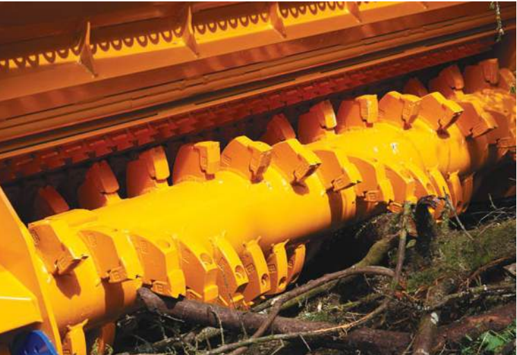
Fixed hammers Options available. Suitable for managing wooded areas and providing a chipped wood finish. Benefits are mulching the debris within the soil leaving the ground level.
