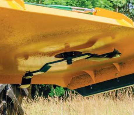
Blade carrier Fitted with updraft blades.
