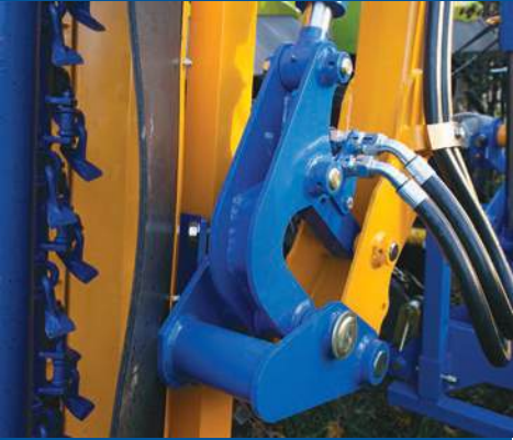
240° cowl bracket linkage For a greater angle range.
