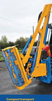
As a result of the 110° power slew the Osprey has a compact inline transport position.
