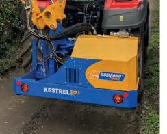
**Power slew and hydraulic breakout** For driver and machine safety.
