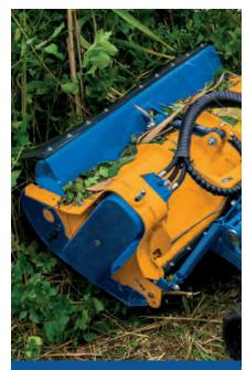
Hydraulic front hood Operational via controls with electronic interlock for safety dependent on rotor direction.
