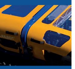
Integral rollbar Standard on all Flailbot models, and offers the additional feature of lift points.
