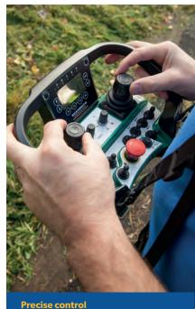
The remote control, operating all Flailbot functions has a range of 150m (492').
