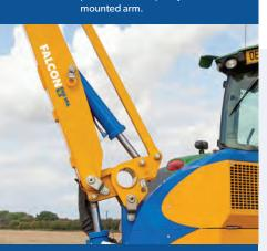
Parallel linkage Comes as standard to assist operator control.
