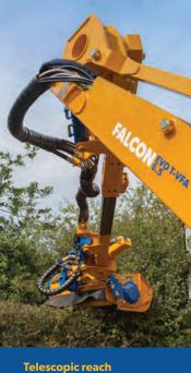
The VFA allows total flexibility of position during arms operation.
