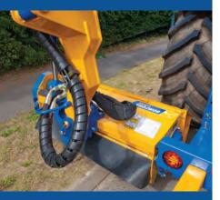
Close in ground cutting Variable arm technology allows forward and rearward reach, enabling cutting in behind the tractor wheel.
