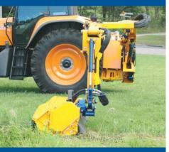
Forward reach position 900mm (35"). Enables midmounted head position with simplicity of rear mounted arm.
