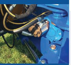
**Powerful 100L hydraulics** For continuous use. Twin pumps with separate oil tank.
