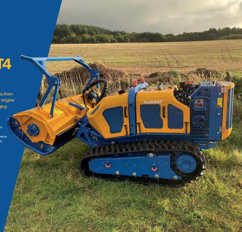
Excellent grip characteristics Individual tracks can be extended by up to 250mm (10").
