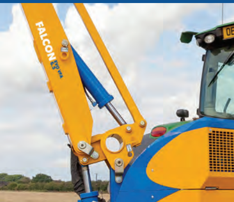
Parallel linkage Comes as standard to assist operator control.
