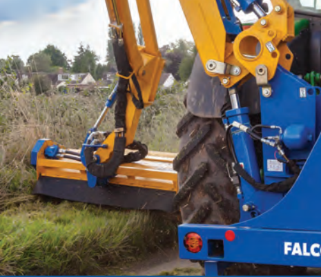
Arm float cylinder To aid grass cutting on roadsides.
