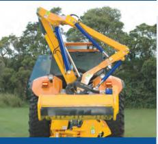
**Transport position** Folding 3rd arm allows compact transport position.
