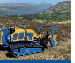
Excellent grip characteristics Individual tracks can be extended by up to 250mm (10").
