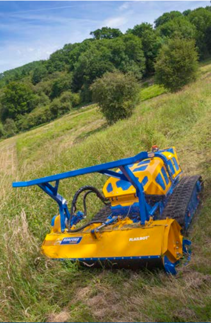
Shredding head Fitted as standard with 1650mm (5'5") shredding head and pushbar.
