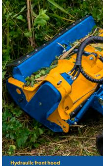
Operational via controls with electronic interlock for safety dependent on rotor direction.
