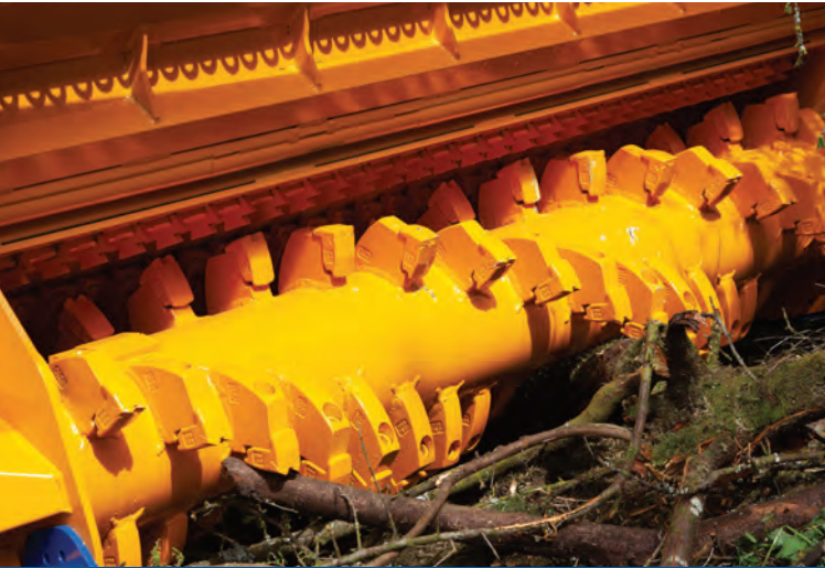
Fixed hammers Options available. Suitable for managing wooded areas and providing a chipped wood finish. Benefits are mulching the debris within the soil leaving the ground level.
