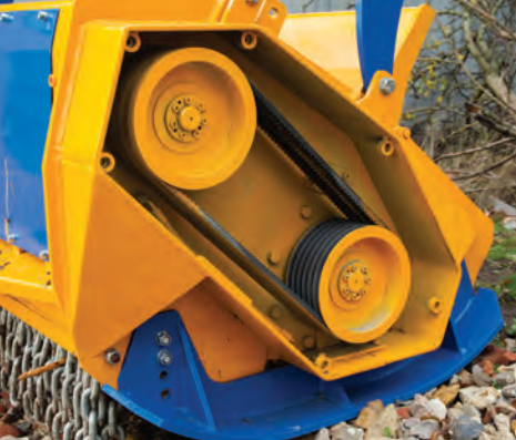
Heavy duty drive 5 belt drive on SD models and 8 belts (dual drive) on HDX ranges.
