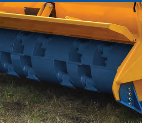
Swinging hammer options Ideal for use on green vegetation for shredding.
