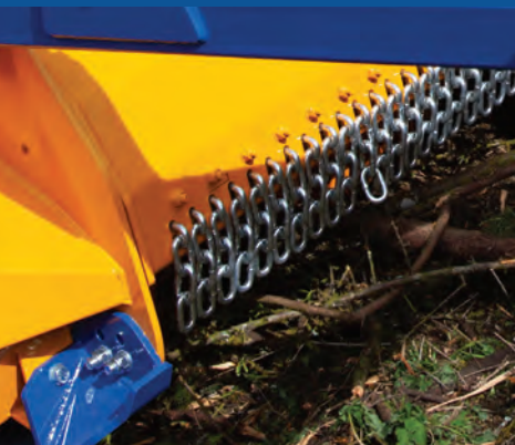
Protection Double rows of heavy chains and adjustable skids.
