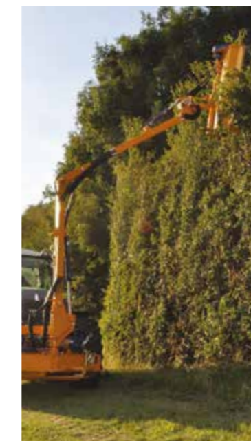
Telescopic second arm On the B58FM T model.
