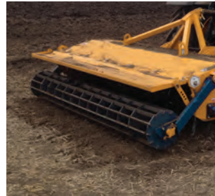
Crumbler Roller Break down soil clods to give a fine finish ready for drilling.
