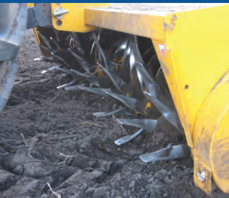
Front rotor Tines lift soil and turns into rear rotor to break down soil structure.
