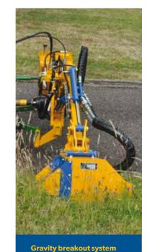
For protecting drive and machine during operation.
